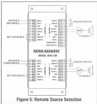
Remote source selection: Figure 5 shows a way of remotely selecting one of two program sources to feed a number of rooms. Rooms 1 and 2 can select between music source A or B. Using a 4082-CM, six rooms can have independent remote selection of two program sources.
